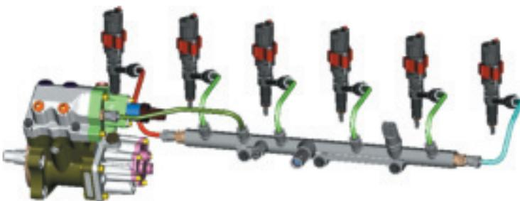
With full-authority electronic control of injection timing, this new level of combustion efficiency by Cummins enables NOx emissions to be reduced by almost 40% to meet Tier 3/Stage IIIA standards. A higher degree of combustion control combined with fuel injection precision also allows these engines to quickly and easily handle increasing load demands more rapidly.
