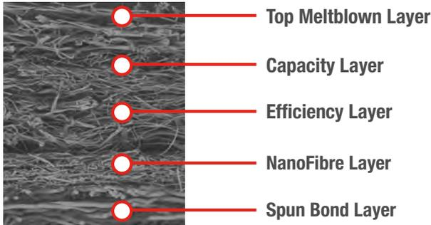
This microscopic view of NanoNet media shows how five distinct layers of protection capture and trap particles in a mesh no thicker than a 10c piece. Once contaminants are trapped in this multi-layered matrix, they can't escape.
