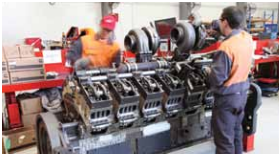
Fit-up of valve train, fuel and exhaust systems.
