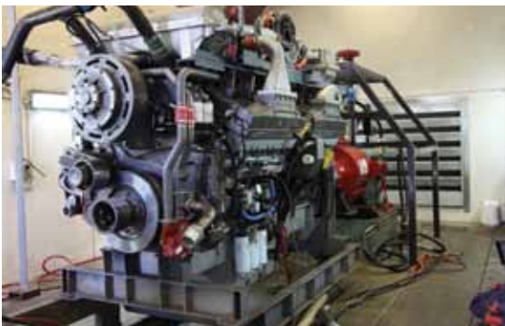
Dynamometer test facilities are capable of testing engines up to 4000 hp.
