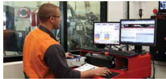
Dynamometer control centre.
