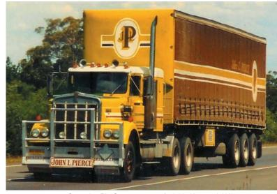
Cummins Big Cam 350 propelled this Kenworth W900.
