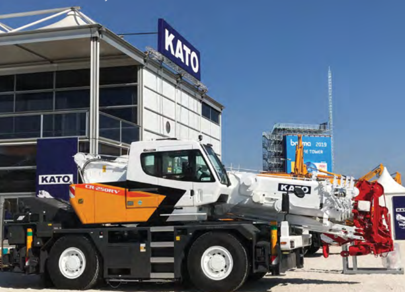
New 25-tonne capacity CR-250RV Cityrange crane powered by the Stage V Cummins QSB6.7 rated at 205 kW (275 hp) was displayed at Bauma this year.
