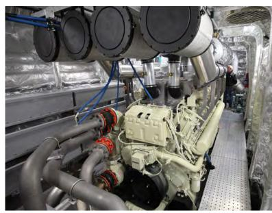
3,600 hp QSK95 fitment in Kilimanjaro VII exceeds Cummins' installation requirements, reflecting high build quality.
