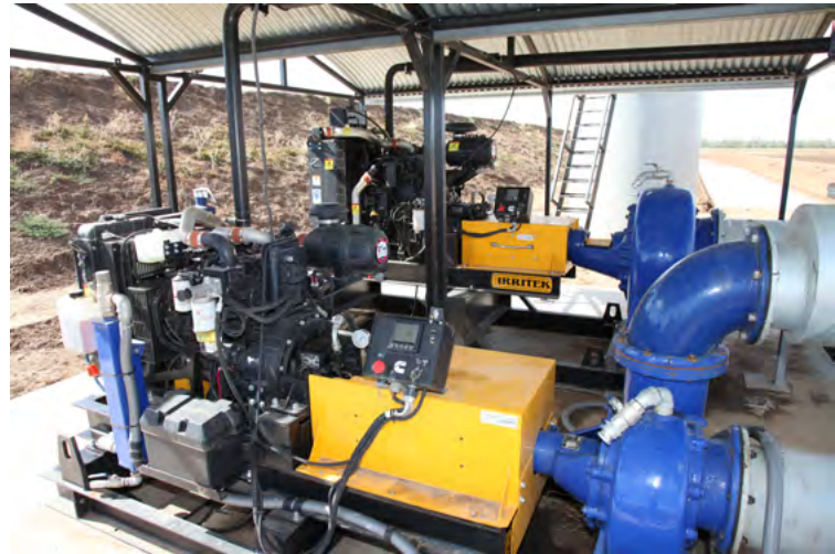
The latest Cummins engines at CSD Farms are electronic Tier 3 QSB3.3 and QSB4.5 units which are proving their fuel efficiency.
