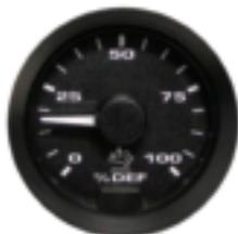
The Low DEF lamp illuminates and stays on continuously when the DEF level is low. A flashing DEF lamp indicates that the DEF level has fallen below the critical level.
