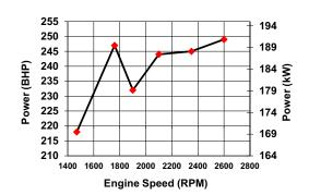
All data is based on the engine operating with a fuel system, water pump, lubricating oil pump, air cleaner, and alternator. The fan, optional equipment, and driven components are not included. Data is based on operation at SAE standard J1349 conditions of 300 ft. (91.4 m) altitude, 29.61 in. (752 mm) Hg dry barometer, and 77 °F (25 °C) intake air temperature, using No.2 diesel fuel only.
